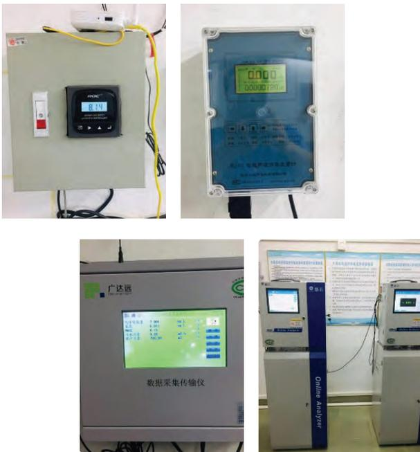
Photo 2 Sewage pollutants monitoring devices installed in Zhongshan factory
