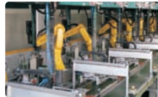
Avoiding production of dust with automatic wet processing robotic arms
