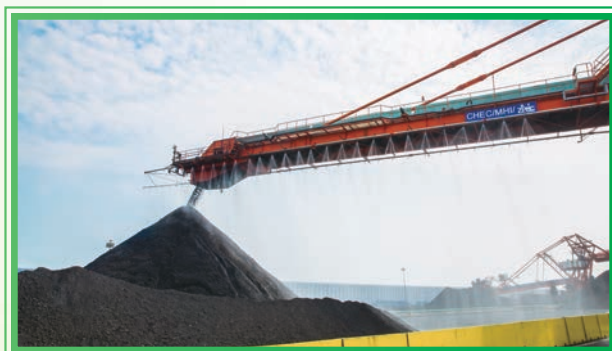
Dust treatment in Huanghua Port – water sprinkled from the Arm of Stacker
